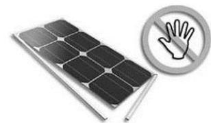
Do not apply paint or adhesive to the top surface of modules.
